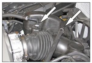
3. Release the grey locking tabs securing the crank case vent and oil tank vent tubes to the factory intake hoses and then disconnect the crank case hoses from the intake tube.
