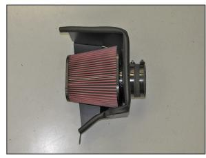
17. Set the air filter into the heat shield and then install the provided coupling hose (08761) onto the filter and secure with the provided hose clamp.
