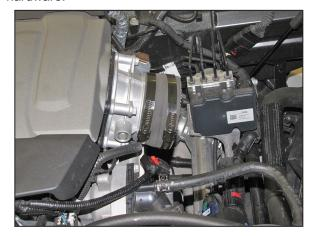
19. Install the provided coupling hose (08761) onto the throttle body and secure with the provided hose clamp.
