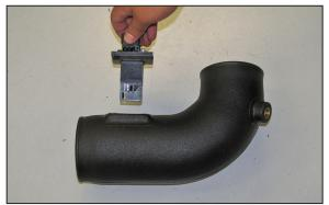
23. Install the mass air sensor assembly into the K&N® intake tube and secure with provided bardware
