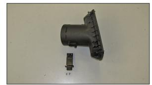
20. Remove the two screws securing the mass air sensor to the factory housing and then remove the sensor from the housing.
