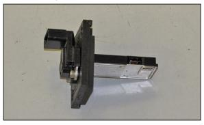
22. Install the mass air sensor into the provided adapter and secure with the provided hardware.
