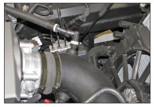
26. Connect the crank case vent hose to the fitting installed into the K&N® intake tube as shown.
