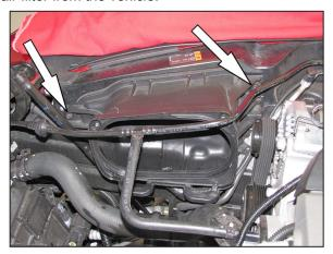
8. Remove the two bolts that secure the air filter housing to the inner fender then unhook the housing from the mounting stud and remove the housing from the vehicle.
