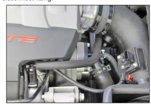
31. Reinstall the 90° quick disconnect fitting onto the valve cover port and then connect the open end of the hose to the fitting installed into the K&N® intake tube.
