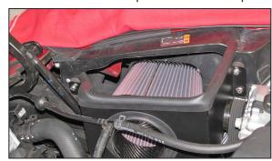
18. Install the heat shield assembly onto the rubber mounted studs and secure with the provided hardware.
