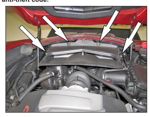
2. Remove the four bolts that secure the air extraction duct to the radiator and then remove the duct from the vehicle.
