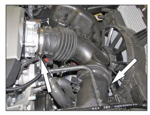
6. Loosen the hose clamps that secure the factory intake tube to the throttle body and air filter housing and then remove the factory intake tube from the vehicle.
