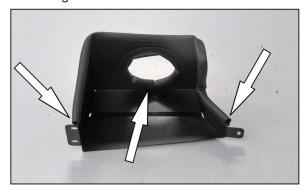
16. Install the 16" section into the hole of the heat shield and install the 27" section around the perimeter of the heat shield as shown.
