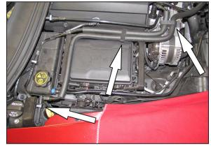
4. On vehicles that are equipped with a "Dry Sump" oiling system, release the grey locking tap securing the oil tank vent hose to the oil tank, then unhook the oil tank vent hose from the two retaining clips and remove the hose from the vehicle.
