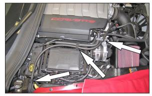
28. On vehicles that are equipped with a "Dry Sump" oiling system, install the crank case vent hose assembly onto the oil tank and then route it through the factory retaining clips and then connect the open end to the 90° fitting installed into the K&N® intake tube.
