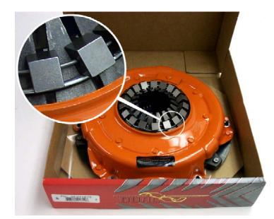
Dual Friction clutch assembly is designed to provide a positive engagement with daily drivability. Install the Dual Friction disc with side indicating "Flywheel Side" against the flywheel (typically the segmented or puck style facing as shown.)
