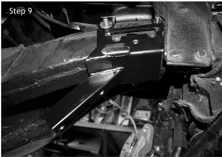
9. The driver's side bracket slides up from the bottom. The lower bolt hole uses a 3/8 x 4" long bolt. Install this bolt now.
