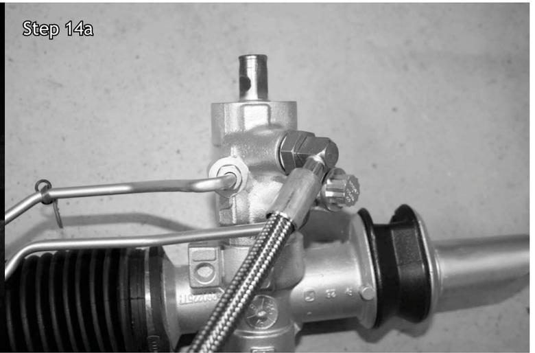
14. Install the braided return line on the top rack port nearest to the pinion (the smallest hole). Now install the rack and pinion on the brackets using the supplied clamps and 5/16 x 1" bolts, washers and nuts. Please note the 2 rack clamps provided are shaped differently - they must fit properly on the rack. Torque the pass. side bolts to 30 ft-lbs but leave the driver side loose until completing step 17.
