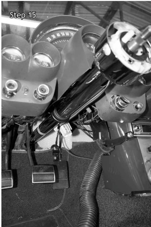
15. Now install the steering column by sliding the small end through the firewall from the inside of the car. First plug in the supplied wiring harness to the column and the corresponding connectors on the car. Use the original column clamp to secure the column to the dash but do not completely tighten until the following step.
