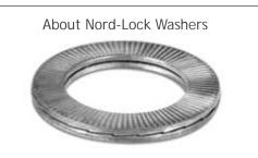
NORD-LOCK is a pair of washers with a wedge-locking action meeting DIN 25201 which is a unique method using tension instead of friction. The rise of the cams between the NORD-LOCK washers is greater than the pitch of the bolt. In addition, there are radial teeth on the opposite side. The washers are installed in pairs, cam face to cam face.
