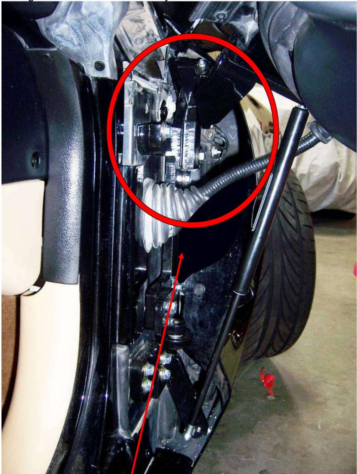
Drill new hole for support bracket.. use M6x1 bolt.
