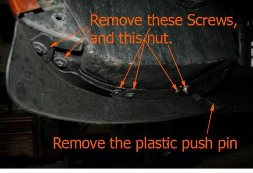
careful removing this pin because you could rip the rubber center
