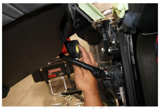
Use zip tie to secure the 2 half of the wire boot to the wire loom as show.
