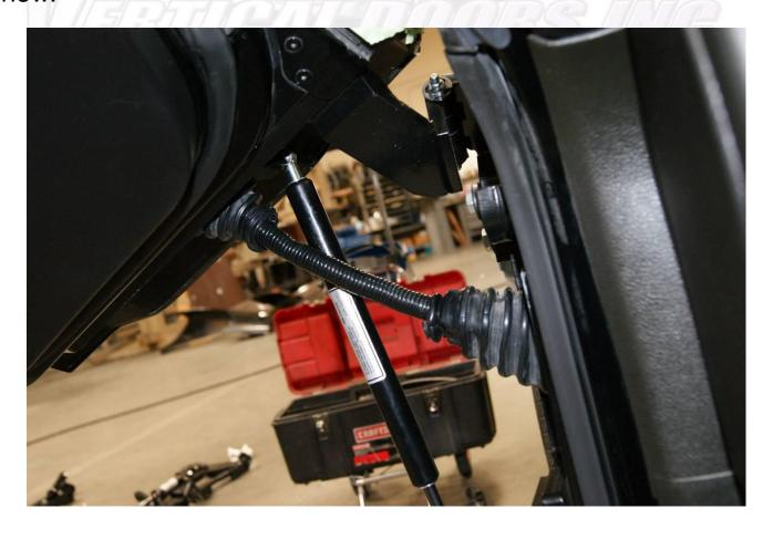
Cut the inner lip of your fender to make room for the new ZLR Door kit..Note: this picture is for reference only you may not need to cut as much on your particular vehicle.. all you need to cut is just enough for the kit to move freely.
