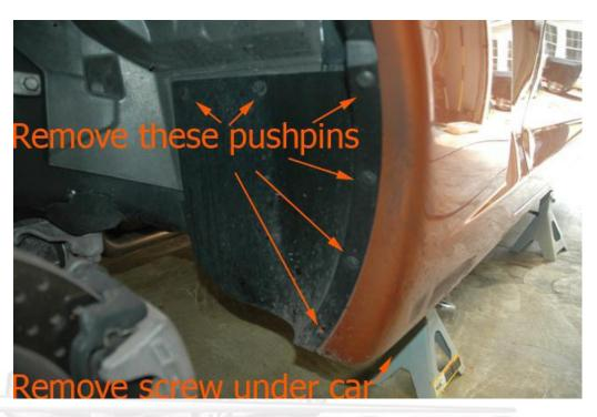
Remove brake dust assembly
