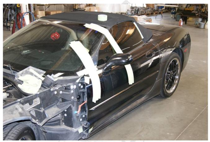
After making sure you have the factory location marked use several strips of 2" painters tape to secure the door to the vehicle.
