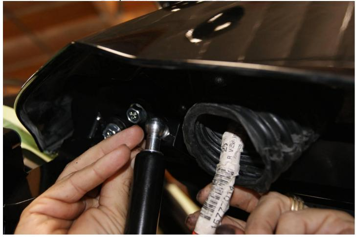
After the kit is installed you can now make the fine tuning adjustments. You will need an Allen wrench for the first adjustment point. This will allow you to make the striker close like factory by moving the back of the door up or down as needed.
