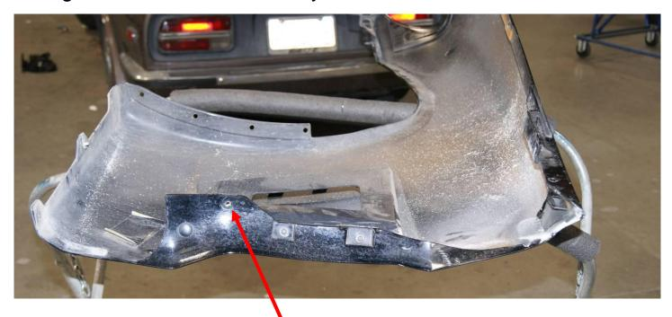
Drill new hole for support bracket.. use M6x1 bolt.
