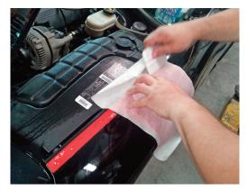
5. Move the stripes into position and use a squeegee or a credit card and gently smooth out the air bubbles.
