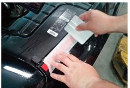
3. Apply the alignment stripe starting at the top of headlight as shown. Use a squeegee or a credit card to smooth out the air bubbles.
