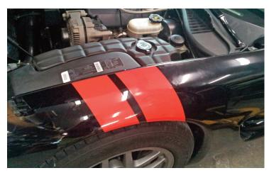
9. Use a squeegee to remove any bubbles of fluid under the decal. If you have some small bubbles that you cannot remove don't worry, the decal does breath and fluid will evaporate after a couple of days. If it is a must that you have the bubbles removed you can use a pin to puncture the decal and squeeze out the fluid.
