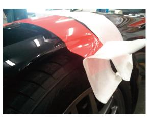
6. When the stripes are in place, remove the transfer tape without pulling up the stripes. If the stripes start to come off, squeegee back into place and let decals dry a few minutes longer.
