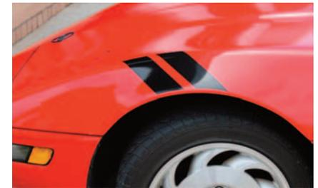
6. Use a squeegee to remove any bubbles of fluid under the decal. If you have some small bubbles that you cannot remove don't worry, the decal does breath and the fluid will evaporate after a couple of days. If it is a must that you have the bubbles removed you can use a pin to puncture the decal and squeeze out the fluid.
