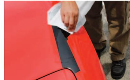
5. Once you have removed the tape you can remove the alignment tags from the fender of the car.
