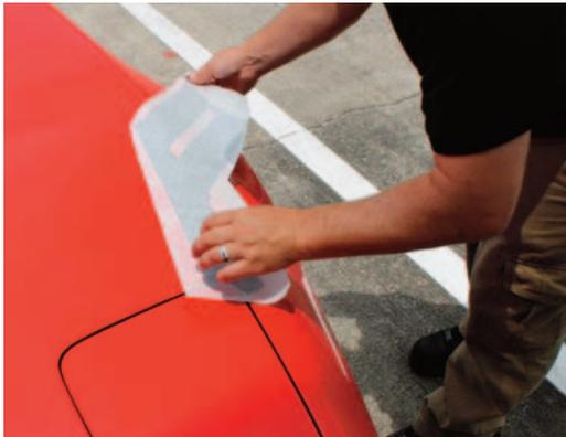
3. Apply the decal starting with the alignment tags from the top of the headlight as shown.
