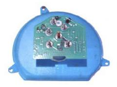
Remove the three nuts that retain the tach board to the tachometer. This is done with a 5/16" nut driver.
