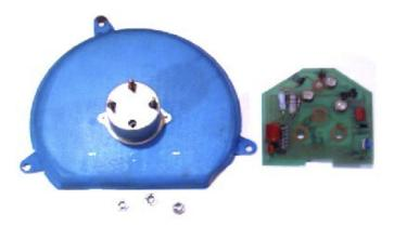
The new board may look a little differently than the one you are replacing. This should not be cause for concern. The new board will come with three new fiberboard red insulators not used on the original board. You should have the parts show below once you receive your new board.
