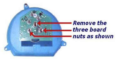
Remove the old tach board and sit the nuts off to the side.
