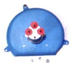
Once you have the insulators on the back of the tachometer, install the new board over top of them as shown.
