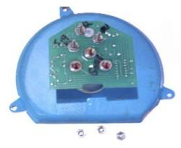
Attach the three board nuts as shown below and you are now finished.
