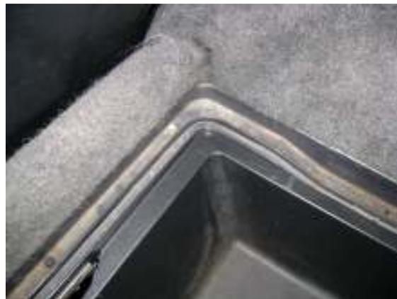
After removing the trim, the rear back wall cargo carpet is held on by some push in clips, which after removing these clips, allows the cargo floor carpet to be pulled out. The wheel well carpet is easily removed when the roof storage bracket trim is removed, as well as the speaker grilles.
