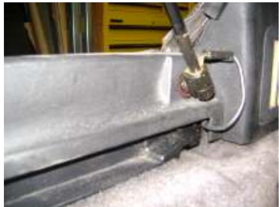
***NOTE: You will need to remove the roof top storage release latch handle, and the screws in the cargo cover rails to remove the trim panels, and remove the rear carpet easier.***
