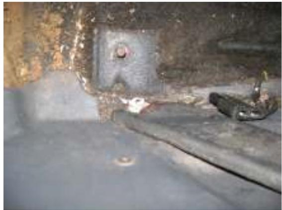
Be sure to remove the door sills, including the e-brake cover, before removing the floor carpeting. With the seats and console removed, the front floor carpet comes out easily.
