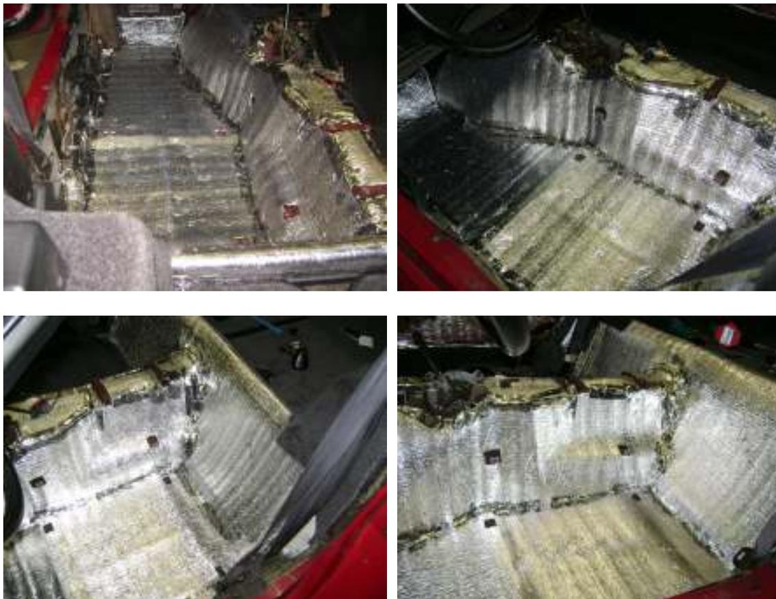
Go ahead and tape the edges of the floor piece down, and then lay out every other piece where it is labeled to go. This helps to see what areas are covered, and where the seams are that need to be taped.
