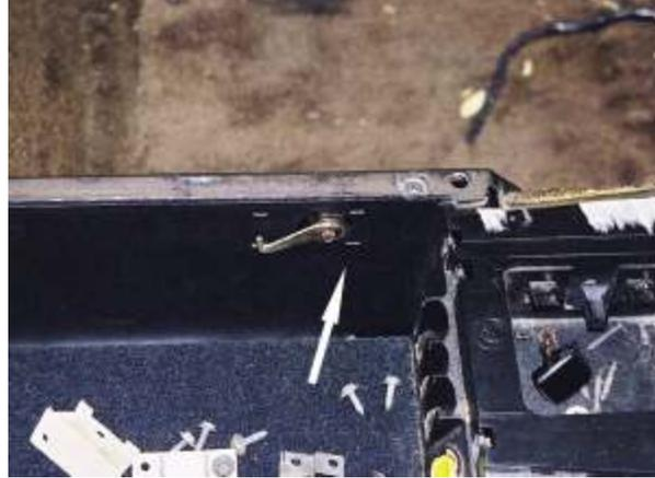
After removing the center console bezels, and the lock assembly, remove the 7mm bolts at the top edge of the center console, as shown below.
