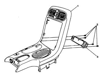
10. Remove the cup holder assembly from the plate assembly instrument panel accessory trim.
