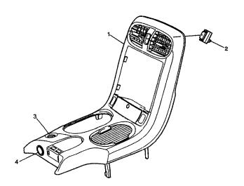
Remove the ashtray from the plate assembly instrument panel accessory trim.
