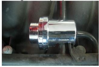
**TECH TIP:** Before placing the end bezel apply a small dab of instant adhesive to the two chrome halves to bond them to each other this will help keep them in place long term. Allow some time for the adhesives to set.
