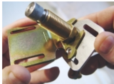
(Fig 30) Slip the tips of the open end of the Pivot Shaft Orientation Bracket onto the brass Pivot Shaft.
