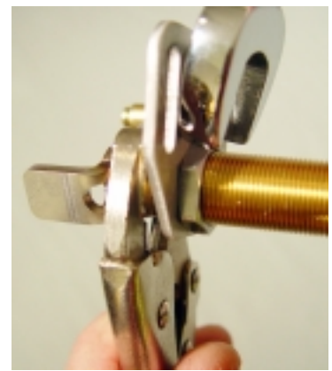
(Fig 23) When running the 5/8-24 hex nuts down the barrel of the Pivot Shafts, it may help to hold the brass shaft with pliers or vice grips and use a 3/4" wrench.
