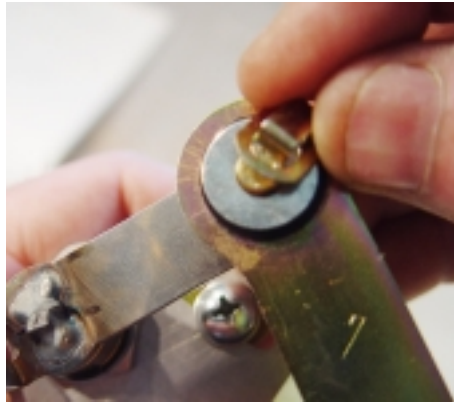
(Fig 92) Place a thin washer and spring clip onto the exposed end of the upper brass pivot pin on the Drive Unit.
