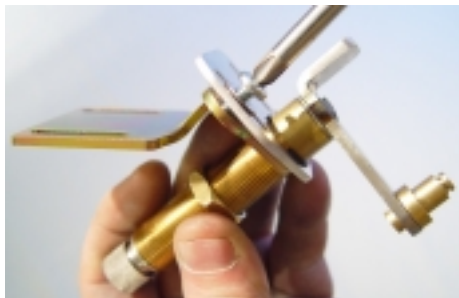
(Fig 32) Using two 10-32x3/8" phillips head screws and flat washers, attach the aluminum Pivot Shaft Holding Plate to the Pivot Shaft Orientation Bracket.
