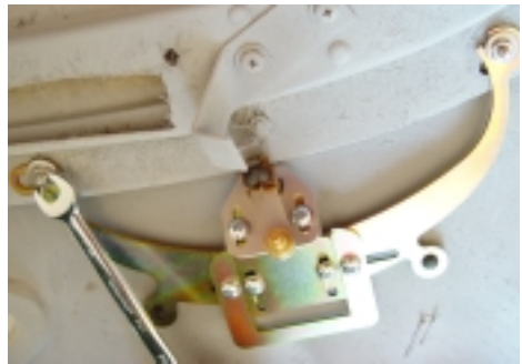
(Fig 76) Place #12-24 hex nuts and 1/4" flat washers on the windshield retaining studs and tighten them.
