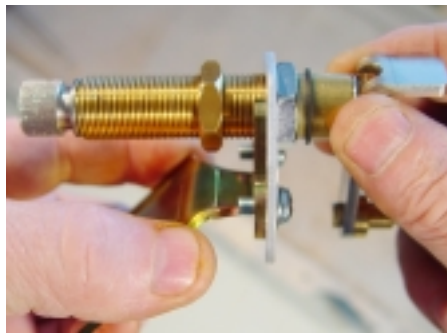
(Fig 82) Loosen the 5/8-24 hex nut closest to the tip and rotate it toward the tip by the distance you want to pull the tip closer to the cowl.
