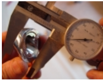
(Fig 10) The early escutcheons are about 1.06" in overall depth.
