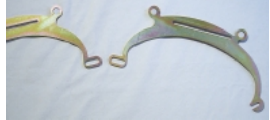
(Fig 13) Place the two Pivot Shaft Mount Plates on a table with the tips with slotted holes touching.
