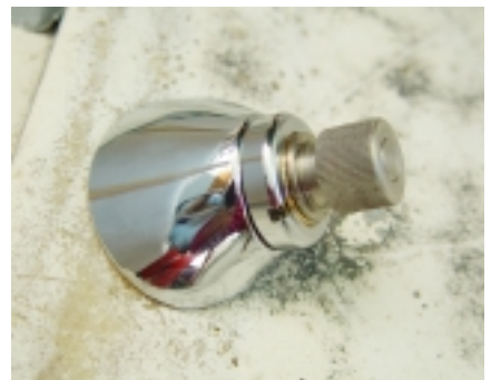
(Fig 84 & 85) When you are satisfied with the fit of the Pivot Shaft and chrome escutcheon fit on the outside of the car, tighten all interior screws before installing the chrome escutcheon nut with the aluminum Escutcheon Wrench supplied in the kit. Overtightening can damage the fiberglass.
