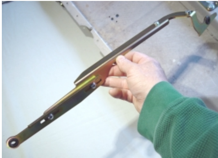
(Fig 50) Attaching the Corner Stiffener to the passenger side Link.
