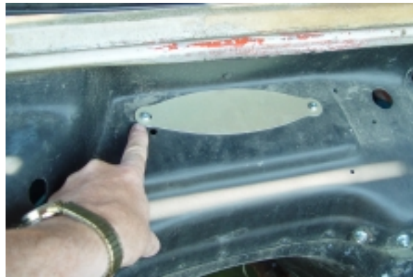
(Fig 102) The Cover Plate goes where the old motor was mounted.
