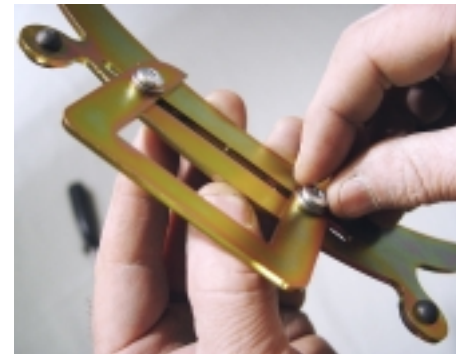
(Fig 16 & 17) On the opposite side of the pivot shaft Mounting Plate, the 4 nut backing strip is used to attach the "U" Guide to the Mounting Plate.
