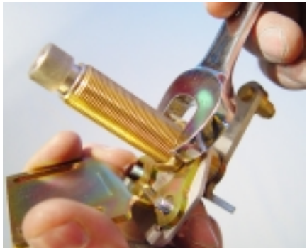
(Fig 33) Run the hex nut down to the Pivot Shaft Orientation Bracket about finger tight.
