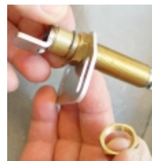
(Fig 16 & 17) On the opposite side of the pivot shaft Mounting Plate, the 4 nut backing strip is used to attach the "U" Guide to the Mounting Plate.
