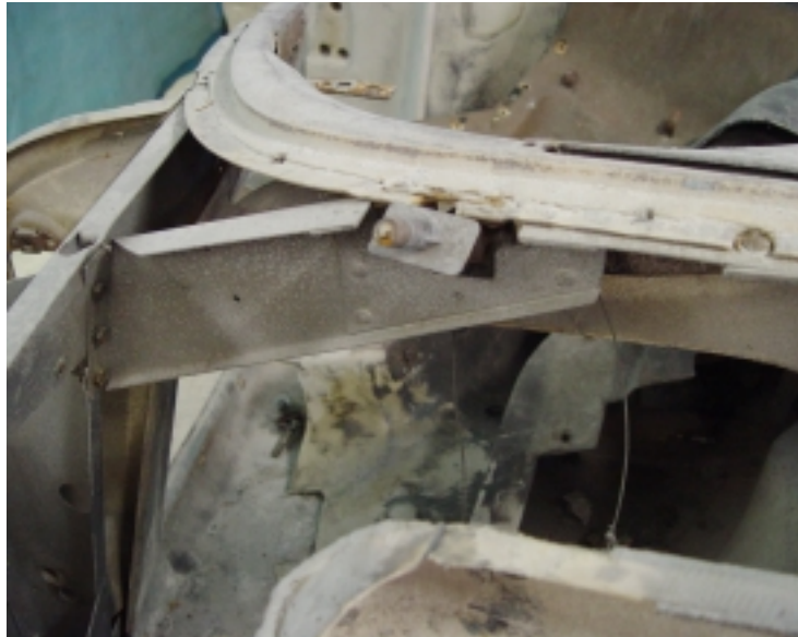
(Fig 70) This is the passenger side looking aft. The fiberglass cowl has been removed. This Corvette has the metal substructure that requires separating the Pivot Shaft Orientation Brackets from the Pivot Shaft Mounting Plates and "U" Guides to install the Pivot Shaft Mounting Plates and "U" Guides between the metal substructure and fiberglass cowl.
