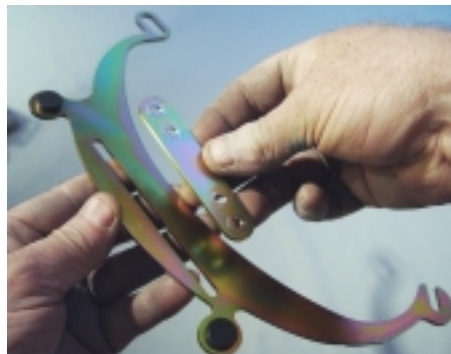
(Fig 16 & 17) On the opposite side of the pivot shaft Mounting Plate, the 4 nut backing strip is used to attach the "U" Guide to the Mounting Plate.
