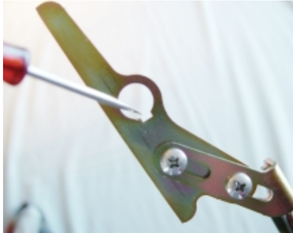
(Fig 63) Push the Plastic Bushing into the keyed hole as far as it will go.
