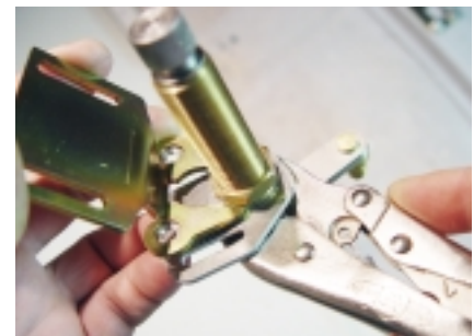
(Fig 31) It doesn't go on the shaft easily. You might find it easier to gently hold the Pivot Shaft with vice grips.
