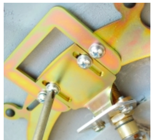
(Fig 78) A primary adjustment is by loosening the four phillips head screws in the Pivot Shaft Orientation Bracket. The inside two give front to back (in and out) adjustment. The outside two give side to side adjustment.
