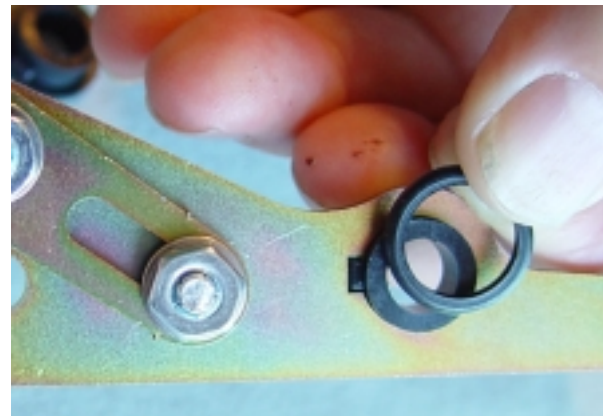
(Fig 64) The Plastic Bushings that fit into the keyed holes in the Link Tips have a plastic ring that fits on the side that extends through the keyed hole.
