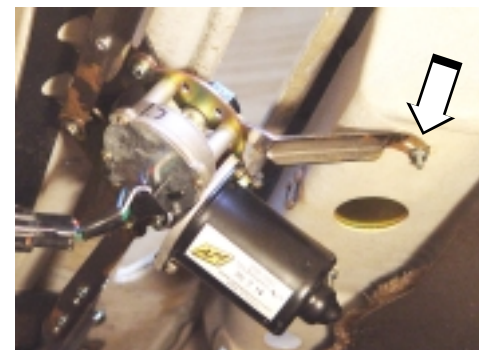
(Fig 45) The opposite end of the Motor Brace goes up against the underside of the firewall where the left side of the old (OEM) wiper motor was attached. Attach the Brace using a 10-32x3/4" phillips, washer, and nut. This same fastener holds one side of the new Cover Plate.
