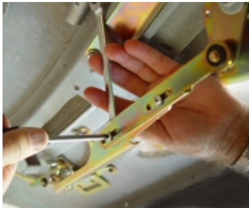
(Fig 96) Driver side Link length adjustment.
