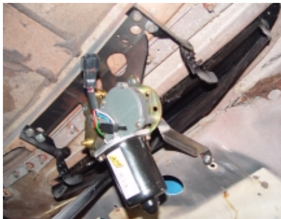
(Fig 44) Place the Main Drive Unit up against the underside of the cowl, between the cowl vent hinge brackets. Use four 1/4-20x3/8" hex bolts and 1/4" flat washers to hold the Main Drive Unit and cowl vent brackets in place.
