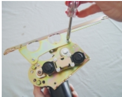
(Fig 40) Using two 10-32x3/8 screws, nuts and washers, attach the motor to the motor mount bracket.
