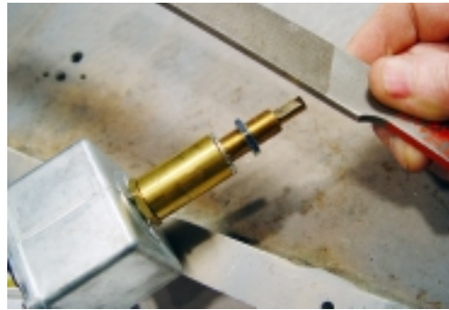
(fig 110) File a flat spot in the shaft at the 6 o'clock position for the switch knob's set screw.
