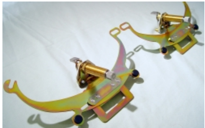
(Fig 32) Using two 10-32x3/8" phillips head screws and flat washers, attach the aluminum Pivot Shaft Holding Plate to the Pivot Shaft Orientation Bracket.
