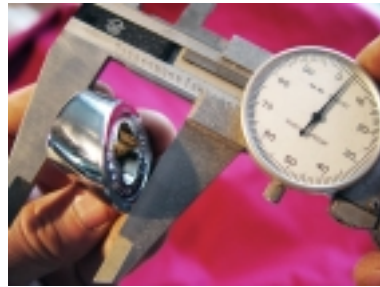
(Fig 12) 1958-62 1.20" chrome escutcheons are identical, both right and left side.
