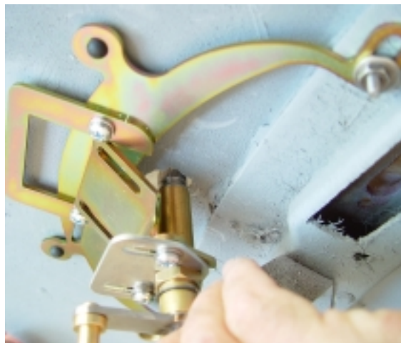
(Fig 74) Insert the Pivot Shaft with the Pivot Shaft Orientation Bracket upward toward the corresponding wiper shaft hole in the fiberglass cowl. This car does not have the metal substructure.
