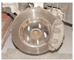
Step 5: Install hub cover to rotor.
