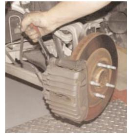
Step 3: Loosen top caliper bracket mounting bolt with 22 mm socket, then remove lower caliper bracket mounting bolt.
