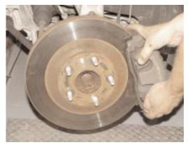
Step 4: Swing caliper out enough to slide hub cover onto rotor. (Do not remove caliper from bracket.)
