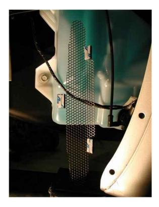
Using a pair of pliers, bend the 3 tabs so they fit flush with the fender outline. Also bend the top section of the grille (area between the two top tabs) Approx 60 degrees in the same direction as the two tabs
