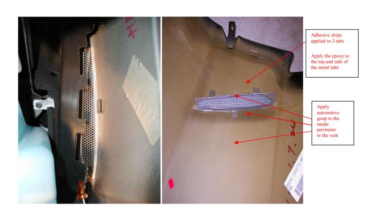
Once you are satisfied with the position of the grille, insuring that it covers the entire open grill area, place a bead of automotive goop or equivalent around the inside perimeter vent opening. Remove the adhesive strips backing and apply.
