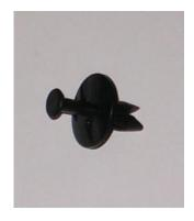
There are several New GM clips that need to be removed. Using a flat head screwdriver, gently raise the head of the clip. Once the head of the clip is raised (releasing the lock), remove the clip. (see picture above)
