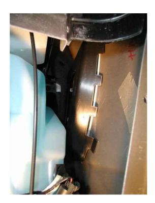
Once you have gained access into the fender area, you will need to remove the inner fender vent box (Black). This box is held into place using double sided tape (2 sections). Just break the tape bonds. You will need to remove a screw mounted to the black box and a bracket. (Mark the area where the tape was mounted, so you can re-install it in the same place.)
