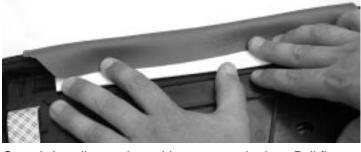
**Step 4:** Install console cushion on console door. Pull flaps firmly securing them to the double-sided tape. (The double-sided tape is intended to temporarily hold the flaps until backing plate is re-installed.) Re-install spring and button and check for operation.
