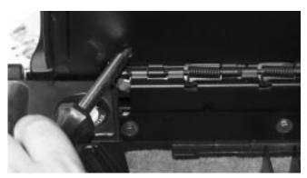
**Step 1:** Remove center console door by removing the screws that secure the console lid to the hinge and unplugging the console light assembly.
