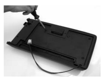
**Step 2:** Lay console lid face down and remove the screws on the plastic backing plate. (84-89 DO NOT REMOVE the 2 screws that hold the light.) Remove backing plate. (Note direction of console lid spring and button for re-installation.)
