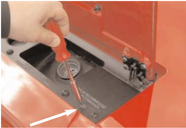
Step 1: Remove the 2 lower screws (or torx) on each side as shown in picture.
