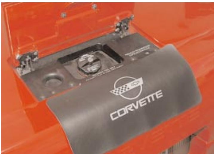
Step 4: Position protector as shown, lining up the pre-punched holes under the assembly to where the 2 lower screws (or torx) were removed.
