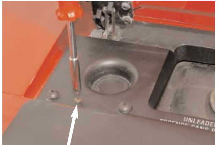
Step 5: Re-install 2 lower screws (or torx) and tighten the 2 top screws.
