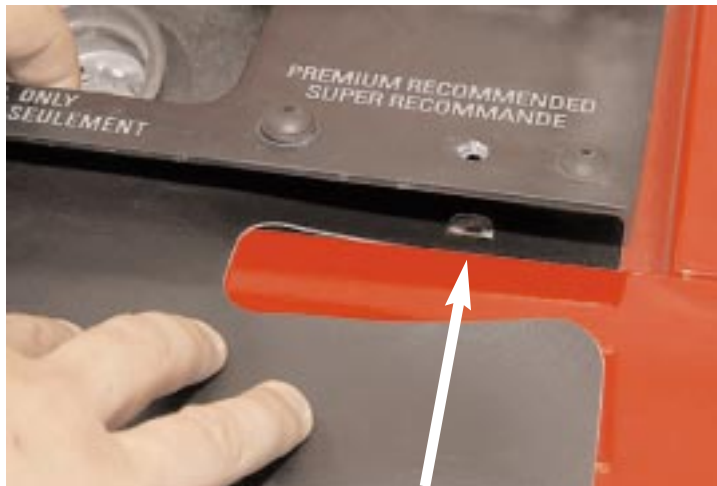
Step 4: Position protector as shown, lining up the pre-punched holes under the assembly to where the 2 lower screws (or torx) were removed.
