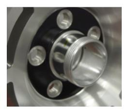
Step 1: Remove wheel from car. (Refer to Service Manual on proper wheel removal). Insert adapter into the front side of the wheel
