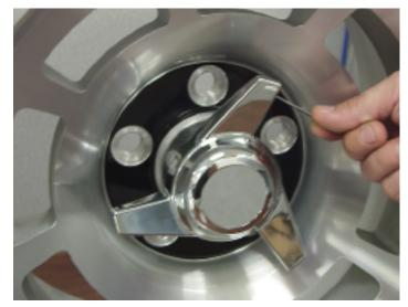
Step 3: Thread wheel spinner onto adapter and secure with set screw to the threaded hole on the back side of wheel spinner.
