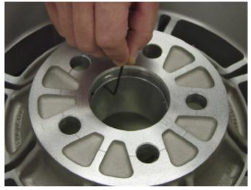
Step 2: Insert 3 set screws in the threaded holes on adapter from the back side of the wheel and tighten securely.
