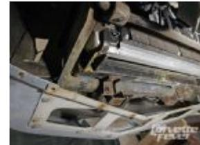
With the baffle removed, a large, open area is created below the radiator. It's easy to see that any air picked up by the spoiler and forced in through the valance will glide right out below the radiator, bypassing it entirely.
