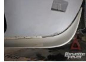
The outer edge of the spoiler may seem a little wide while it's just hanging loose, while there's enough flex to easily bring it in tight with the flowing fender line.
