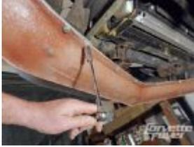
The Eckler's spoiler is predrilled to utilize the factory fastener provisions. We decided not to use the upper baffle to blank the area between the radiator and spoiler as our baffle was in poor condition. To replace it, we'll fabricate a new blanking panel from sheet aluminum later. Start by installing the fasteners just finger-tight so that the spoiler exact position can be adjusted.
