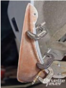
We used some small C-clamps to gently bring the spoiler lip tight to the fender. Don't use excessive force when clamping hard fiberglass.
