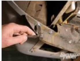
These are obviously not the original fasteners retaining our car's baffle. Years of use have cracked and damaged our stock baffle's mounting holes, with large washers used to hold it in place. The spoiler installation begins by unbolting and removing the baffle.
