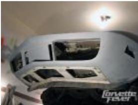
Here's a view under the custom modified fiberglass nose of our '76 Corvette, revealing the stock front lower valance and plastic air baffle. Note the large cooling holes incorporated into the lower valance, and imagine how much air a larger spoiler will force upwards and through the radiator.
